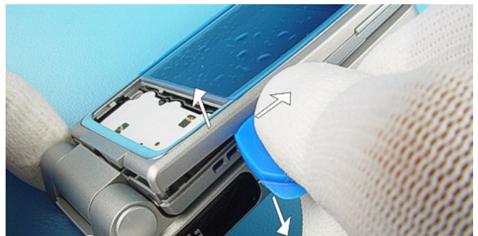
6.) First open the A2 COVER at one side and then...
