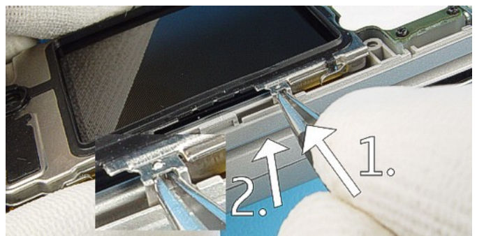
8.) Use tweezers to remove the LCD SHIELD . Start at one side and then...
