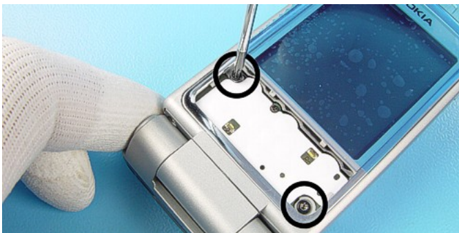
5.) Unscrew the two Torx Plus® size 6 screws. For assembly, a Torx Plus® driver with a torque of 15Ncm has to be used.
