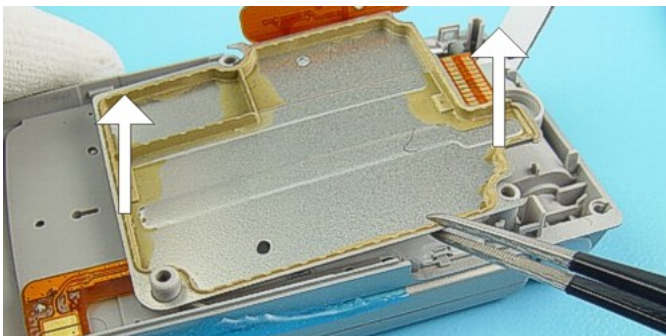
19.) Remove the UI FLEX ASSY by using tweezers as shown in the picture.
