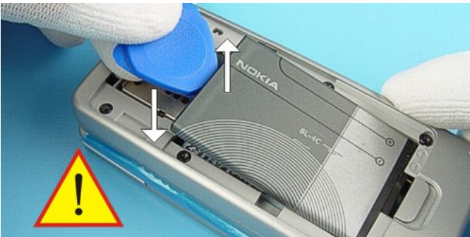
3.) Always remove the BATTERY before continuing disassembly.
