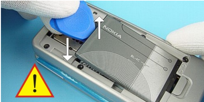
1.) Remove the BATTERY before disassembling the UPPER BLOCK .
