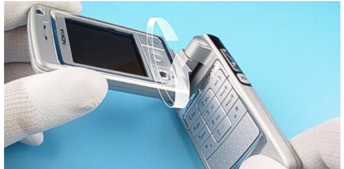
2.) Open the phone and turn around the UPPER BLOCK 180 degrees.
