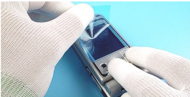
3.) Protect the WINDOW with a film to avoid dust and scratches.
