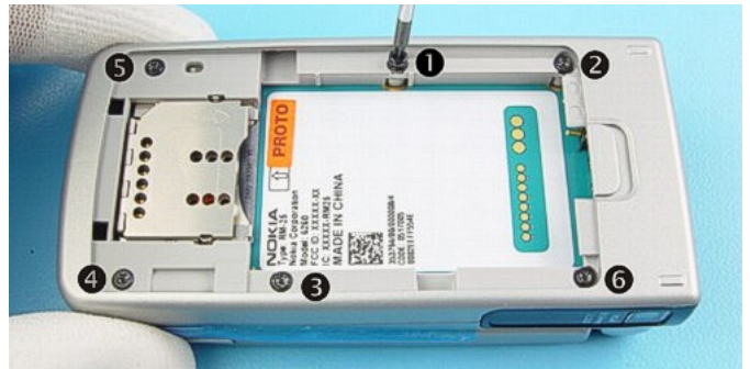
4.) Unscrew the six Torx Plus® size 6 screws. For assembly, the reverse order and a Torx Plus® driver with a torque of 20Ncm has to be used.
