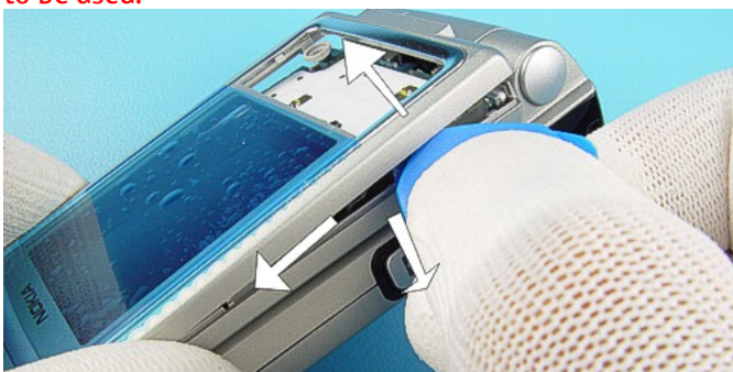
7.) ...at the other side by using the SRT-6 . Remove the A2 COVER .
